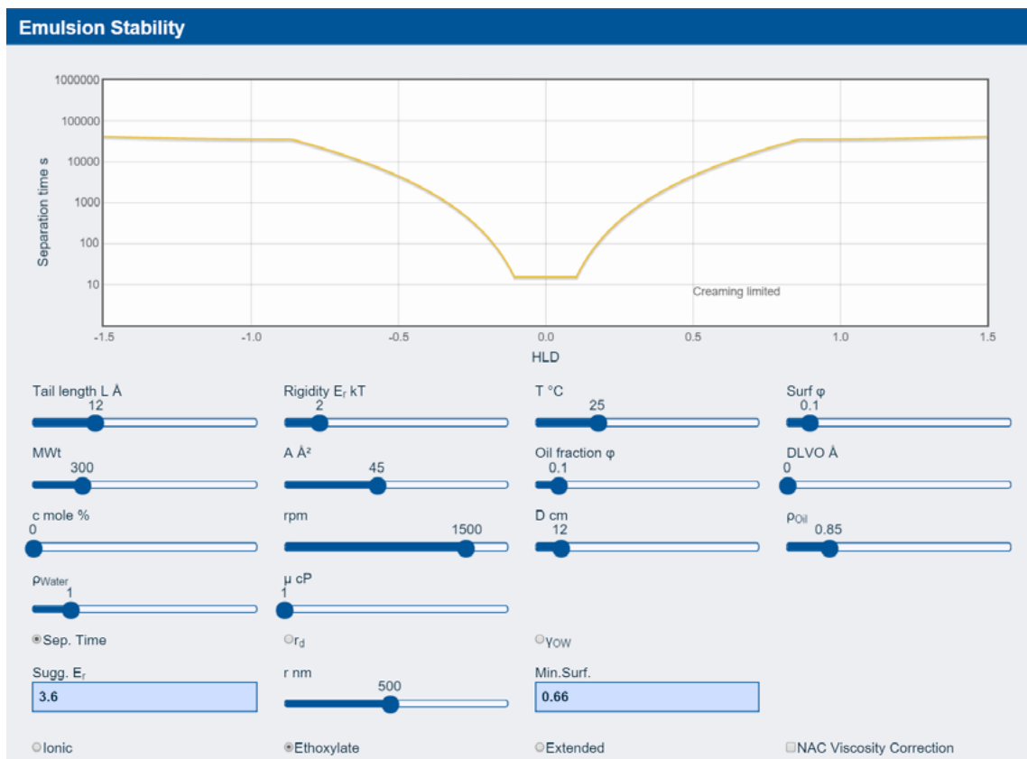
Figure 4-6 The same setup but with oil density set to 0.85. Creaming sets in.
